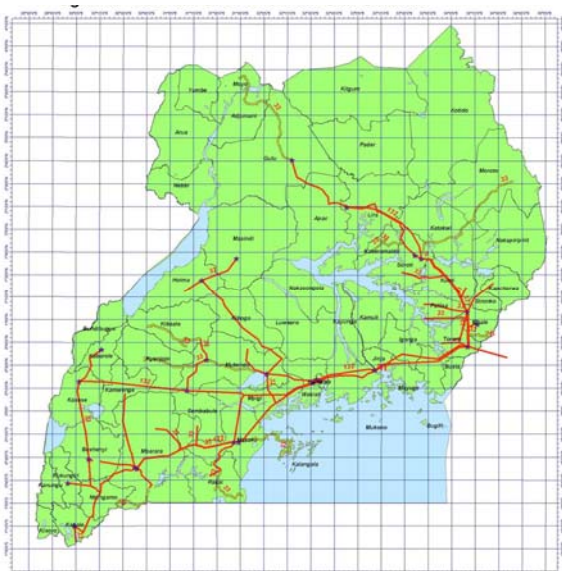
Figure 1: The electricity grid - Transmission Network and some 33kV Distribution lines plus proposed extensions.
